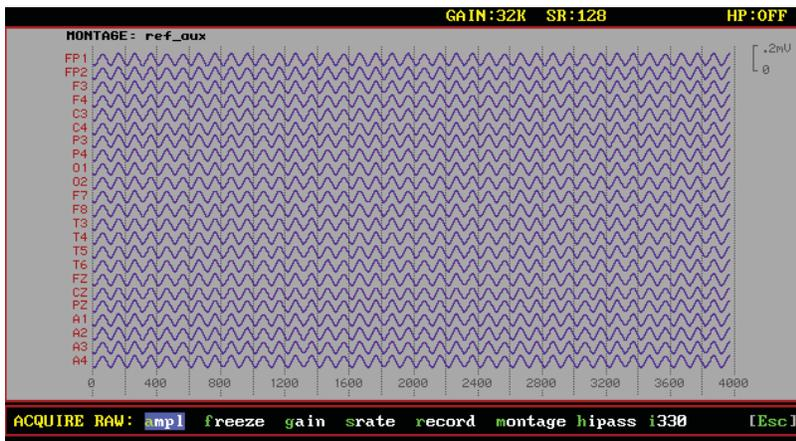
Figure 2. Raw wave display of the 10 Hz calibration signal at 10 microvolts (NeuroLex).
